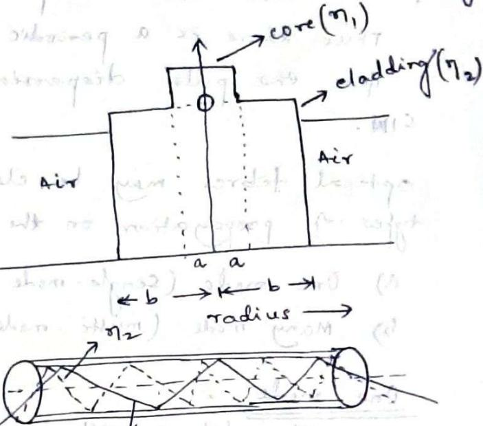
The path length of the ray in air is longer than the direct distance between the two points. The rays travel different path lengths and emerge out at different times.
