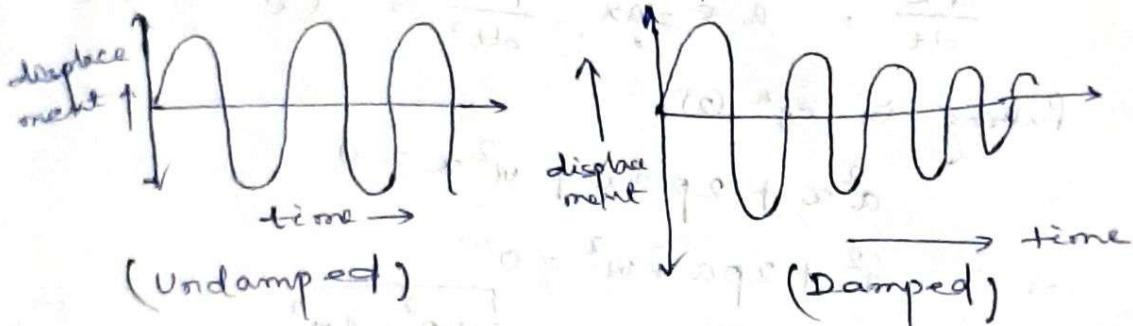
In case of damped vibration, two types of forces act on the vibrating body.
