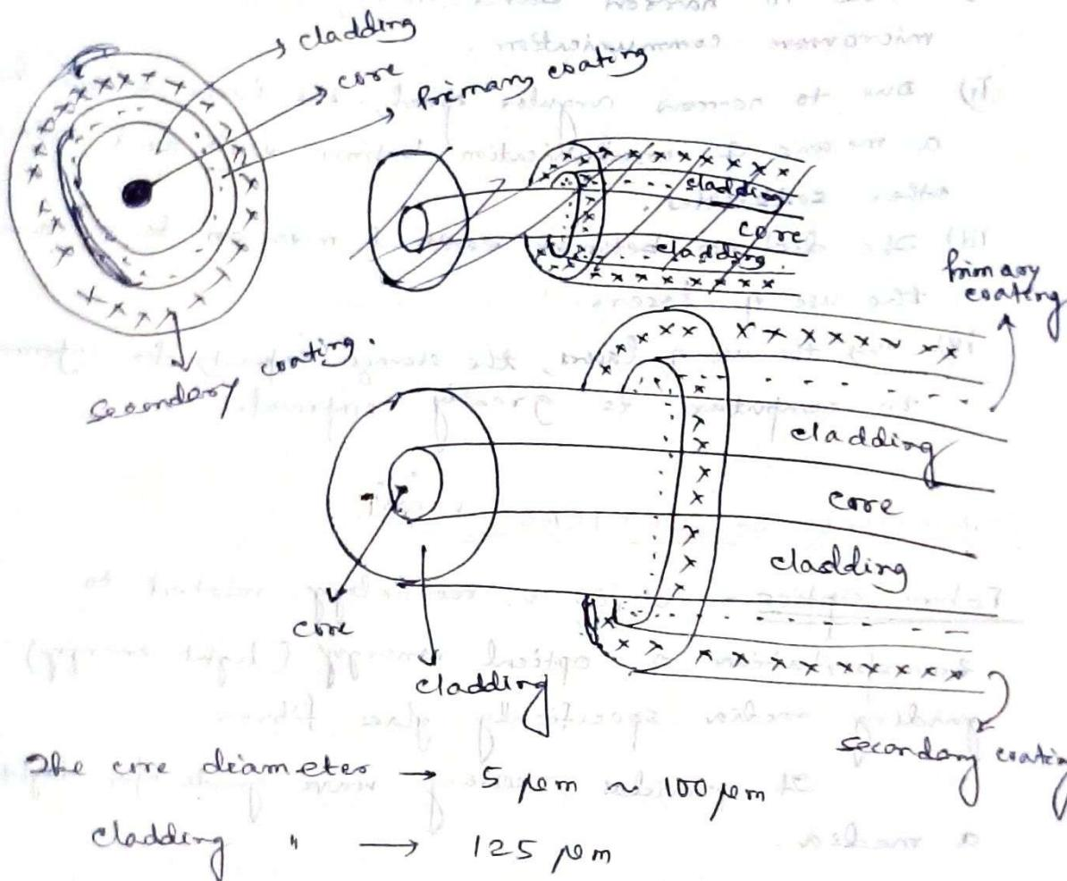
The core diameter  $\rightarrow$  5  $\mu\text{m}$  to 100  $\mu\text{m}$
