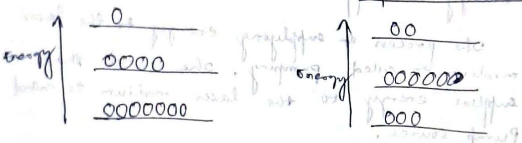
When a population inversion exists, an upper-state system will eventually give off a photon of proper wavelength and drop to the ground state as this photon, however, can stimulate the production of other photons exactly the same wavelength because of stimulated emission of radiation.
