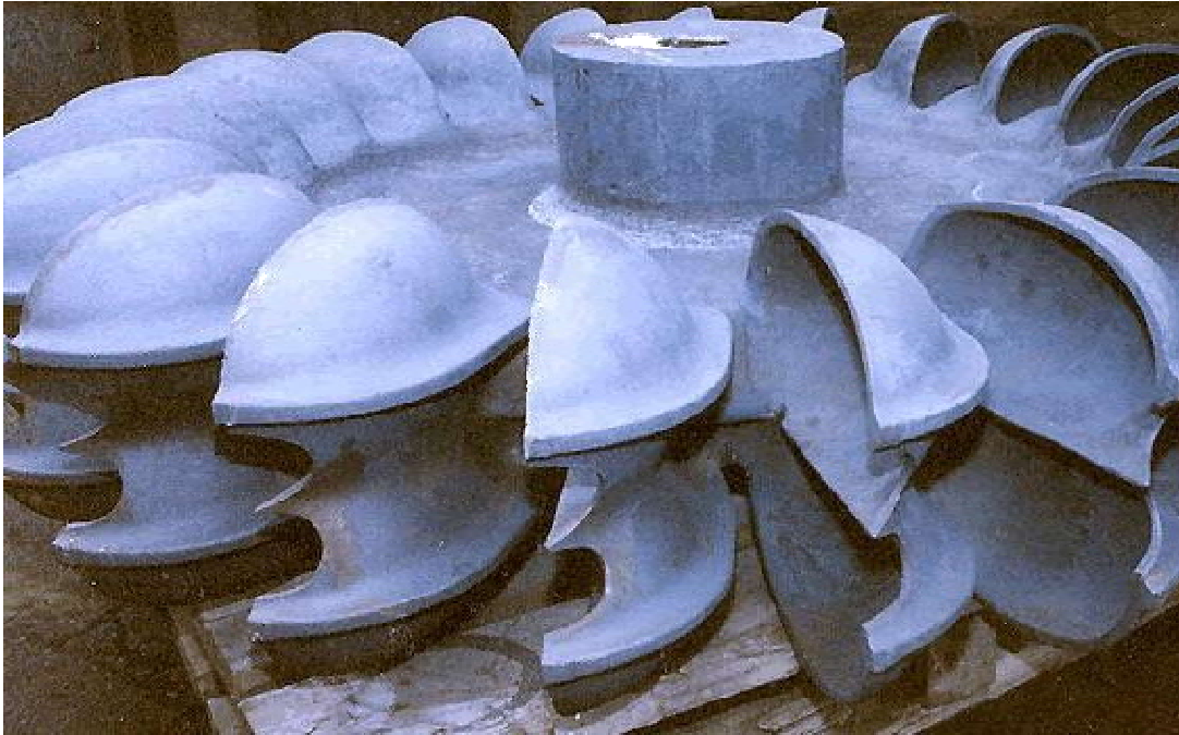
Figure Typical PELTON WHEEL with 21 Buckets
