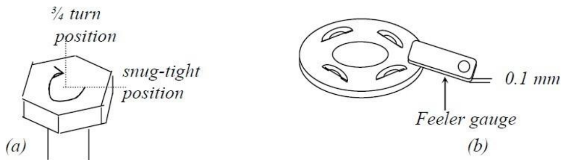
Figure 10.7 Tightening of HSF bolts
