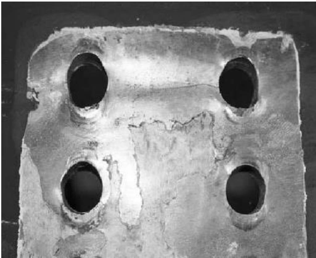
Figure 10.16 Bearing failure of plates
